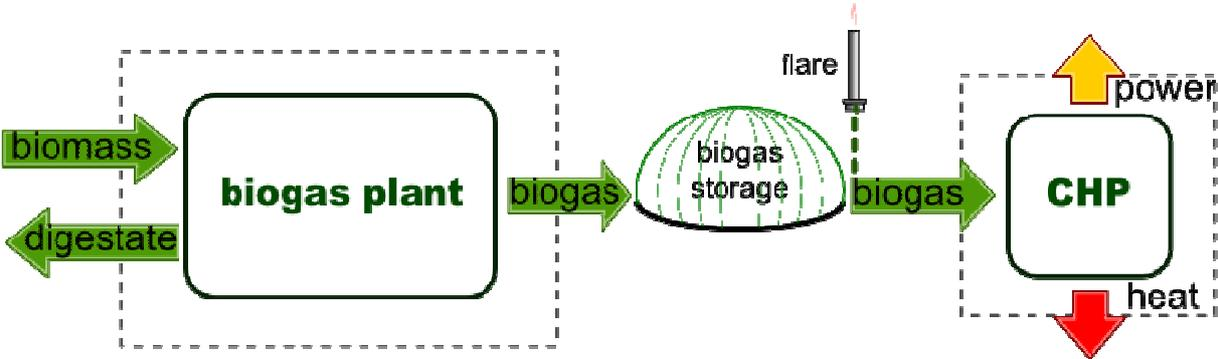
Fig. 1. Simplified diagram of biogas plant with heat and power generation
