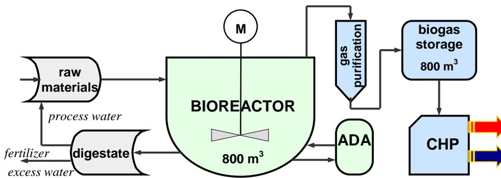
Figure 2.1 Simple flow chart of upgraded biogas plant
