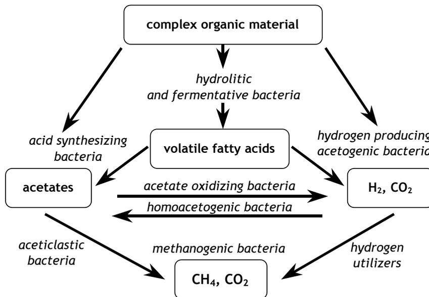
Figure 1.1. Model for the anaerobic digestion process [2]
