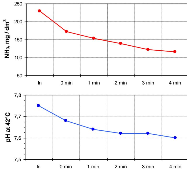
Figure 2.3 Effect of pressurized ADA-treatment on pH and the concentration of free ammonia
